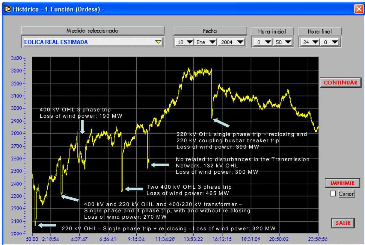
Figure 5.- Spanish wind production during short-circuits (MW)
