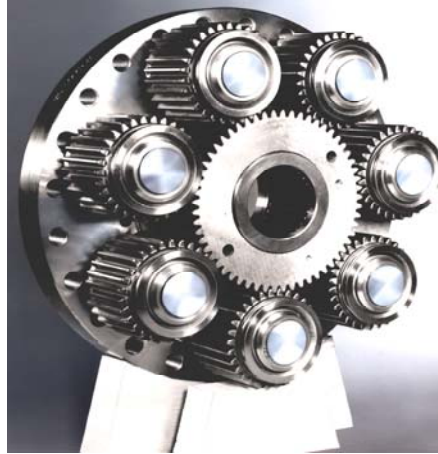
Fig 2 illustrates a typical high speed multi planet Hicks flexible pin planet carrier assembly. The impact of using a flexible pin designed epicyclic train employing maximum number of planets, 7, compared with a conventional rigid three planet design increases the torque capacity a factor of 2.33.
